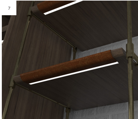
DETAIL: LED Strip Under Adjustable Shelf
